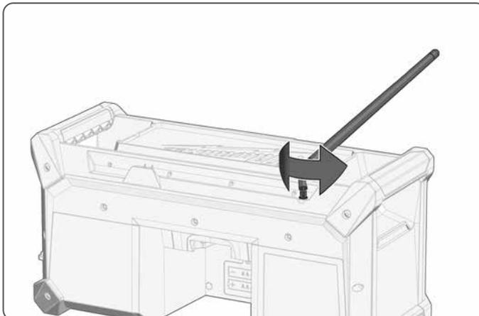
Turn the antenna to different positions/directions for best radio reception. See also chapter "hints for good radio reception" in the text section.
