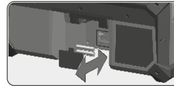
Batteries for backup when battery pack is removed.
