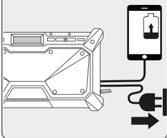
Devices connected to the USB port are supplied with power. Any device that uses more than 3 A of DC electrical current will trip a self-resetting function and disable the output. Charging when the battery is plugged in only when the radio is switched on. When connected to the mains, charging also when the radio is switched off.
